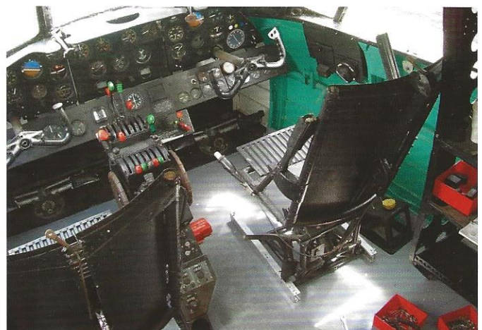
Wolfgang Neumann's hard work has recreated the cockpit of the Viking to include much of the early style equipment.
